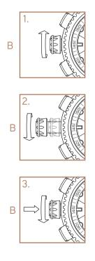
Winding creates the tension required to enable your watch to operate properly.
