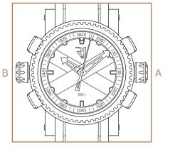
The screw-in crown at 3 o'clock (A) is to set the elapsed dive time controller and the screw-in crown at 9 o'clock (B) to set the time.
