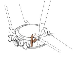
1. Insert the spring bar tool in between the lug and the strap
