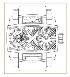
The screw-in crown provide additional protection and increase the case's water resistance. Be sure to never unscrew the crown while under water.
